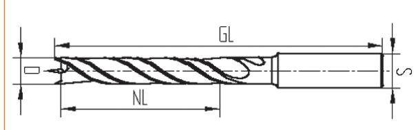
especially for drilling precise holes in soft- and hardwood on portable and upright boring machines etc.
