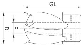
two cutting edges • countersink angle 180° •
