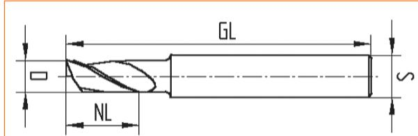
for cutting and milling of aluminium and UPVC profiles etc. on copying machines, water slot milling machines and machining centers e. g. AFS-Schirmer • elumatec • Haffner • Rapid • Rotox • Striffler • Wegoma
