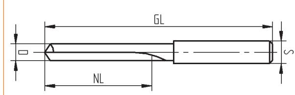
for cutting and milling of UPVC profiles on water slot milling machines e. g. elumatec • Haffner • Rotox • Striffler • Wegoma
