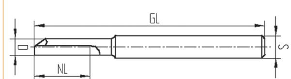
for cutting and milling of aluminium and UPVC profiles etc. on copying machines, water slot milling machines and machining centers e. g. AFS-Schirmer • elumatec • Haffner • Rapid • Rotox • Striffler • Wegoma
