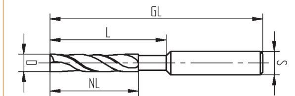
for cutting and milling of aluminium and UPVC profiles etc. on copying machines e. g. elumatec KF 178
