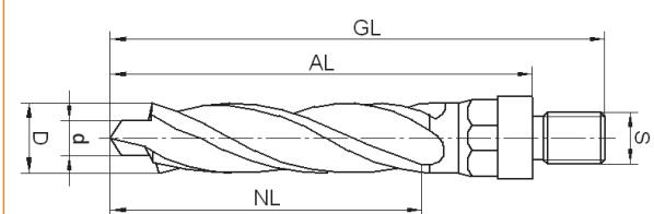
for drilling handles in UPVC profiles with or without steel insert and aluminium profiles on e. g. Ayen • elumatec • Haffner • Mayer • Pertici • Rotox • Striffler
