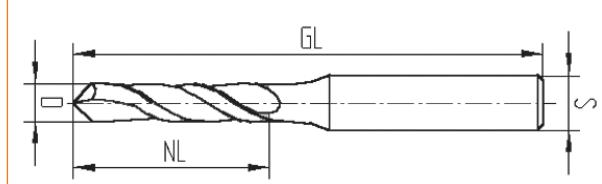
for cutting and milling of UPVC profiles on water slot milling machines e. g. elumatec • Haffner • Rotox • Striffler • Wegoma
