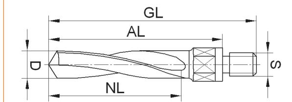
for drilling handles in UPVC profiles with or without steel insert and aluminium profiles on e. g. Ayen • elumatec • Haffner • Mayer • Pertici • Rotox • Striffler
