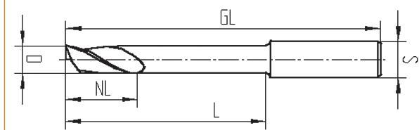
for cutting and milling of aluminium and UPVC profiles etc. on copying machines, water slot milling machines and machining centers e. g. AFS-Schirmer • elumatec • Haffner • Rapid • Rotox • Striffler • Wegoma
