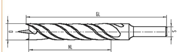
especially for precise inclined drilling (stockade holes) in soft- and hardwood in stair production etc. on drilling attachments for stockade holes e. g. Bohrfix • Bohrluchs
