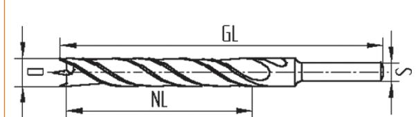
especially for drilling precise holes in soft- and hardwood on portable boring machines etc.
