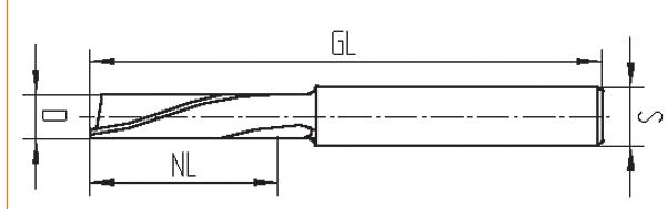
for cutting and milling of aluminium and UPVC profiles etc. on copying machines e. g. elumatec • Haffner • Rapid • Rotox • Striffler • Wegoma
