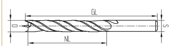
especially for drilling precise blind holes and through holes in soft- and hardwood on portable boring machines etc.
