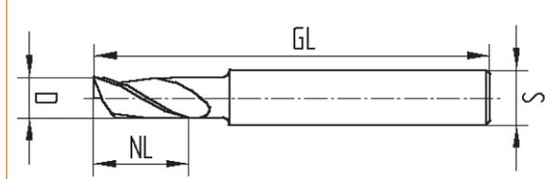
for working steel profiles on copying machines and machining centers e. g. AFS-Schirmer • elumatec • Haffner • Rapid • Rotox • Striffler • Wegoma
