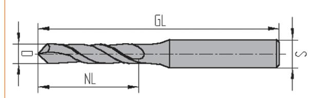
for cutting and milling of UPVC profiles on machining centers e. g. AFS-Schirmer • elumatec • Haffner • Rapid
