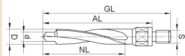
for drilling handles in UPVC profiles with or without steel insert and aluminium profiles on e. g. Ayen • elumatec • Haffner • Mayer • Pertici • Rotox • Striffler
