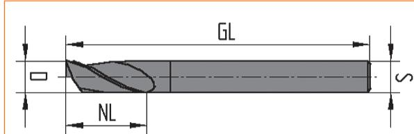
for cutting and milling of aluminium and UPVC profiles etc. on all kind of machining centers e. g. AFS-Schirmer • elumatec • Haffner • Rapid • Rotox • Schüco • Striffler • Wegoma
