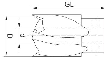
to be used in conjunction with twist drills and dowel drills • for shallow countersinks in soft- and hardwood
