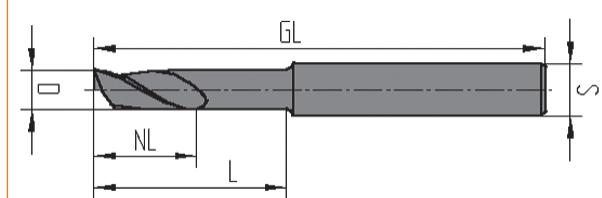
for cutting and milling of aluminium and UPVC profiles etc. on all kind of machining centers e. g. AFS-Schirmer • elumatec • Haffner • Rapid • Rotox • Schüco • Striffler • Wegoma
