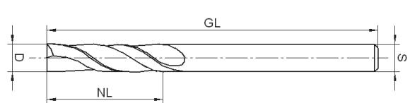
for cutting and milling of aluminium profiles on water slot milling machines e. g. elumatec • Haffner • Rotox
