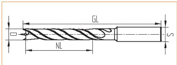
especially for drilling precise holes in soft- and hardwood on portable and upright boring machines etc.
